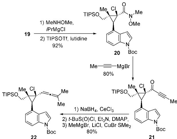
triflate or no reaction when the leaving group was acetate.<sup>15</sup> Eventually, displacement of a sulfoxide leaving group<sup>16</sup> proved to be fruitful and provided the desired allene **22** in 80% yield from ynone **21**.
